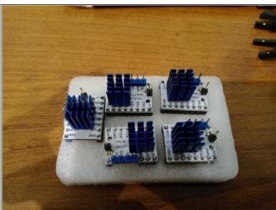
Install the heatsinks delivered with TMC drivers on them as shown on images
