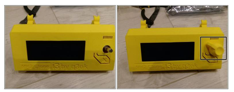
• Put the lcd-knob on the controller
