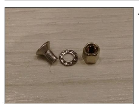
Take 6 sets of pillar, screw and washer from the set with MK42 clone heatbed
